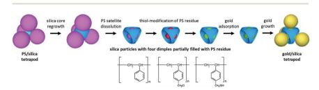
**Scheme 1** Main steps of the synthesis of gold/silica tetrapods from PS/silica tetrapods *via* seeded growth of gold within the dimples.
