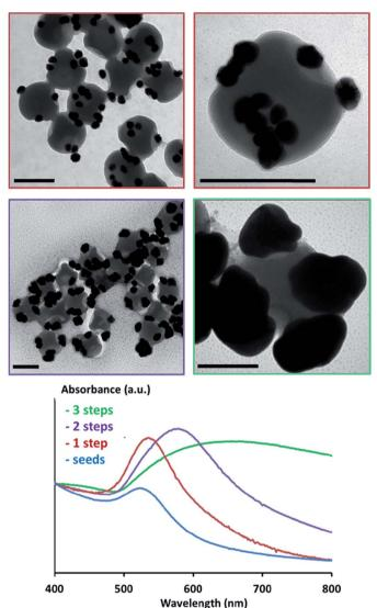
Fig. 5 Transmission electron micrographs and corresponding UV-visible spectra (normalized at 400 nm) of gold/silica nanoclusters obtained after 1, 2, or 3 growth iterations performed in the presence of sodium citrate and ascorbic acid at room temperature. Scale bars are 100 nm.
