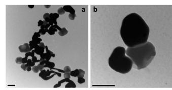
**Fig. 3** Transmission electron micrographs of gold/silica nanostructures obtained after gold regrowth performed in the presence of ascorbic acid and CTAB. Scale bars are 100 nm.
