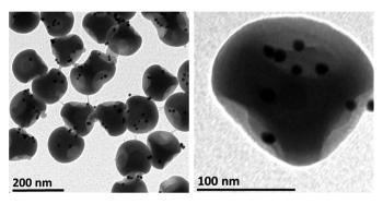
Fig. 2 Transmission electron micrographs of the dimpled silica particles after thiolmodification of the PS chains at the bottom of the dimples and incubation with citratestabilized gold nanoparticles.
