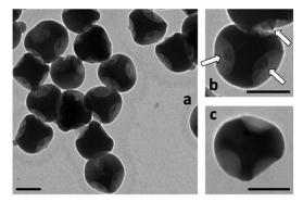
Fig. 1 Transmission electron micrographs of silica particles with four dimples each, obtained from MMS-modified silica seeds (a and b) and from AMS-modified silica seeds (c). White arrows identify polystyrene bumps at the bottom of the dimples. Scale bars are 100 nm.
