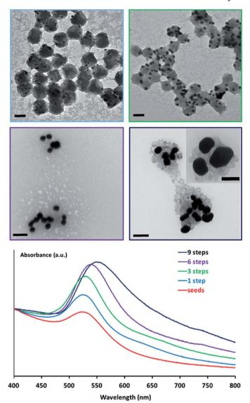
Fig. 4 Transmission electron micrographs and corresponding UV-visible spectra (normalized at 400 nm) of gold/silica nanostructures obtained after 1, 3, 6, and 9 growth iterations performed in the presence of sodium citrate at 90 °C. Scale bars are 100 nm.
