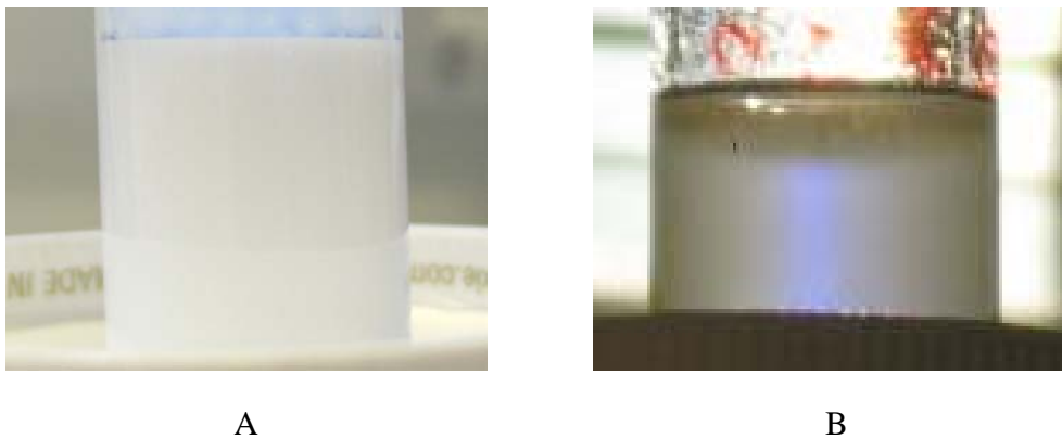
Figure 2: Images of PMMA-co-EGDMA latexes in A) water, B) Toluene.
